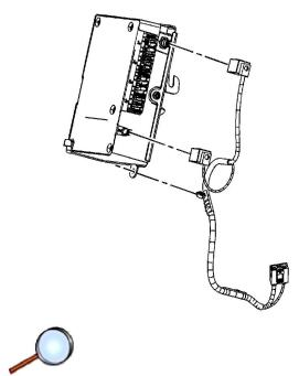
3. Disconnect the VCIM electrical connectors as necessary.
